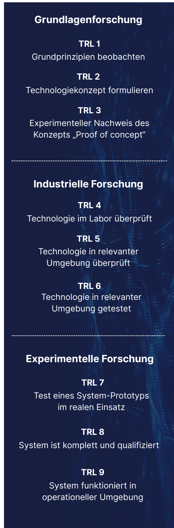
Abbildung 2: Technologische Reifegrade (Technology Readiness Levels (TRL))
